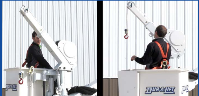
Top mounted jib and winch allows the operator to rotate the jib to work on either side of the rotating basket.
