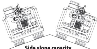
Side slope capacity of -15 degrees horizontal
