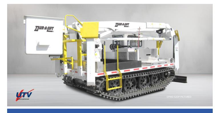
WORKING HEIGHT UP TO 67'; SIDE REACH TO 39'2" MATERIAL HANDLING OR DOUBLE-PERSON TOP OR SIDE-MOUNTED JIB LIFTS UP TO 1000# **180-DEGREE BASKET ROTATOR OPTIONAL BASKET ELEVATOR (DPM2 & DLT2)**
